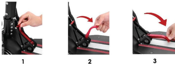
4. Pull also the second folding lever down until the locking mechanism engages (you will hear a click).
