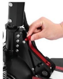
3. Pull the handles upwards until you hear a "click". Then open the quick release clamp and adjust the handlebar height; finally carefully close the clamp.
