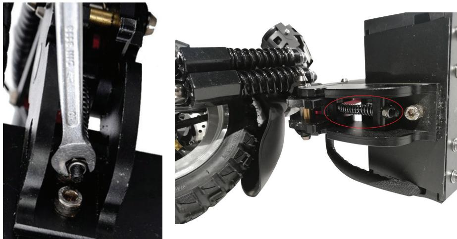
This screw also controls the scooter folding mechanism; if the locking lever is too hard, loosen the nut.
