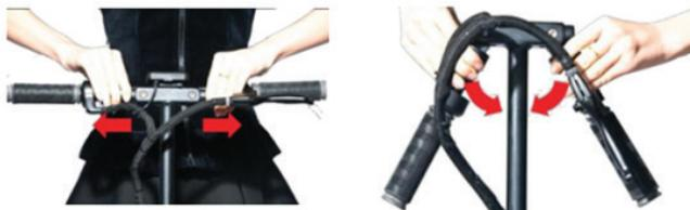
3. Push the first lever down to unlock the folding mechanism;
